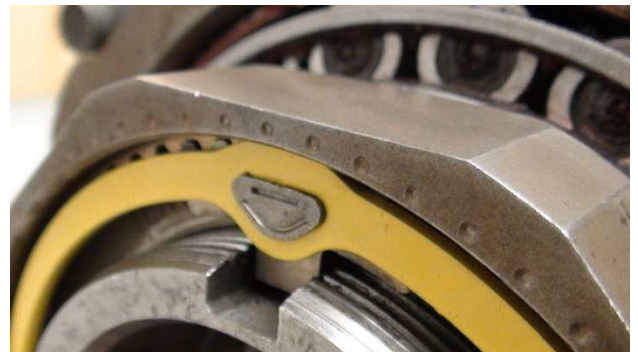
Retainer Tab secured in groove.
