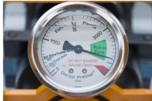
**Do not tighten the Temper-Loc nut against the bearing while the needle pointer is in the green "Roll-In Zone".**
