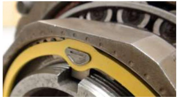
Retainer Tab Inserted Correctly in Nut.
