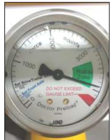
**Do not hand-tighten the Temper-Loc nut against the bearing while the needle pointer is in the green "Roll-In Zone".**
