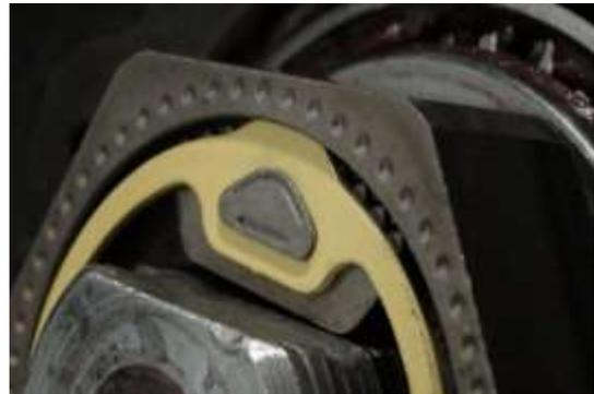
*Retainer Tab secured in groove (FF Style).*
