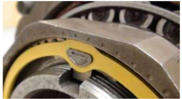
Retainer Tab Inserted Correctly in Nut.
