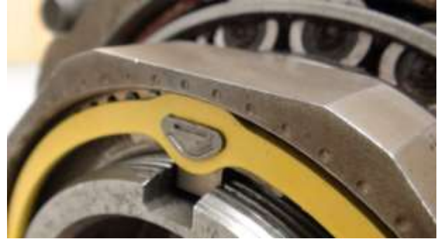
Retainer Tab Inserted Correctly in Nut.
