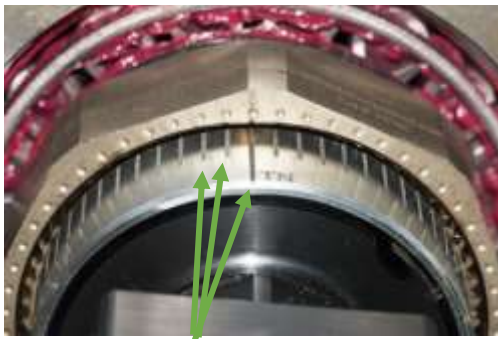
Dots on Nut Face Aligned with Hash Marks on Circular KeyFinder.
