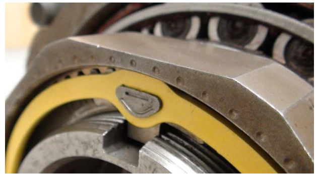
Retainer Tab Inserted Correctly in Nut.
