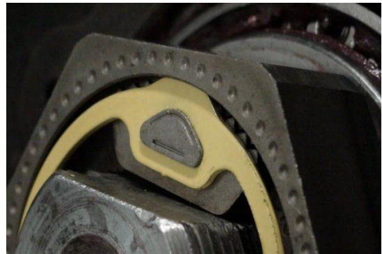
Retainer Tab secured in groove (FF Style).
