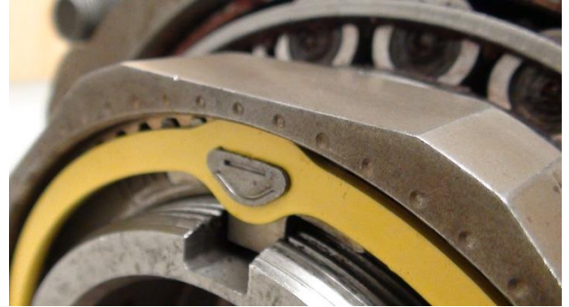
Retainer Tab Inserted Correctly in Nut.
